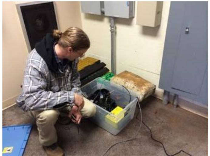
*A USGS researcher installs a seismometer in a building in Washington, DC, to study earthquake ground shaking.*
